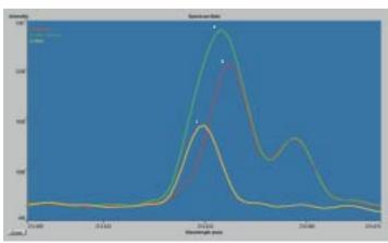
Varian's patented Fast Automated Curve-fitting Technique provides real time spectral deconvolution with no time penalty. **FACT improves** analytical accuracy by solving spectral interference problems in difficult samples. Best of all, if you suspect a spectral interference in your analysis, you can apply FACT after the analysis has finished.
